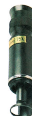
手持显微镜 Microscope T.DL.7582 50X T.DL.7585 75X
